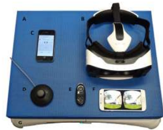
FIGURE 7 | New portable and mobile configuration of the material used in this study: (A) foam rubber; (B) Samsung virtual reality (VR) headset; (C) iPhone running BalancePile App; (D) switch on/off foot button for the Wii Balance Board (WBB); (E) remote controller to launch the visual perturbation; (F) Samsung Galaxy S6 phone running TuscanVista App (visual perturbation); (G) WBB.
