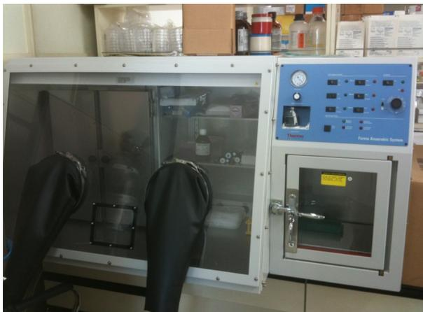
Figure 7. Anaerobic chamber for oxygen-glucose deprivation and reoxygenation
